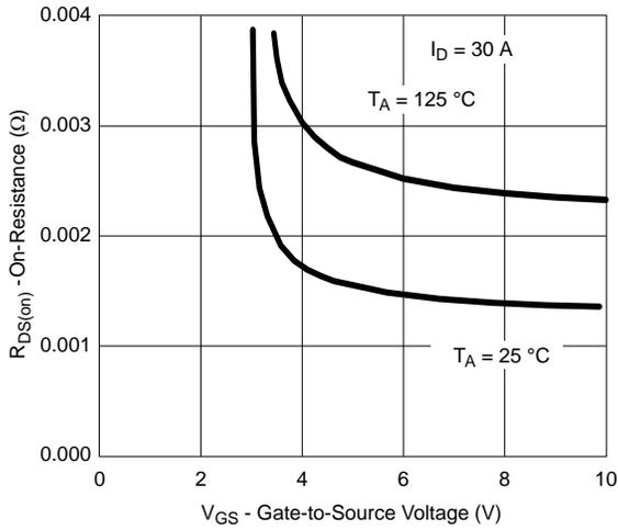
**R<sub>DS(on)</sub> vs. V<sub>GS</sub> vs. Temperature**
