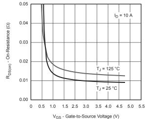
On-Resistance vs. Gate-to-Source Voltage
