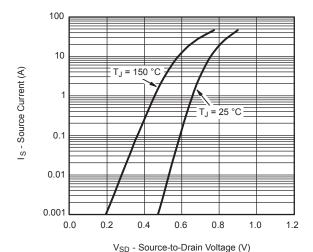
Source-Drain Diode Forward Voltage
